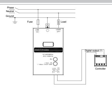
Three-phase Star connection with neutral- GS with VDC control input (Input type "D")
