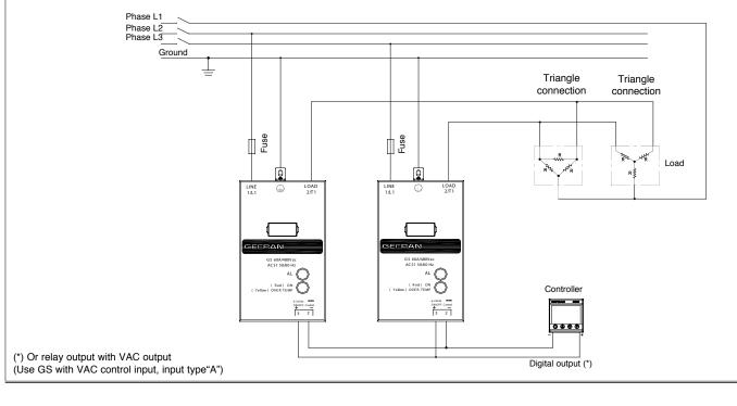
Connection example for GS with VDC control with isolated contact alarm output option (only Models GS-xx/xx-D-1 or GS-xx/xx-D-2)
