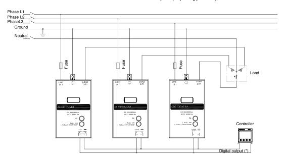
Three-phase Triangle or Star connection without neutral on two phases - GS with VDC control input (Input type "D")
