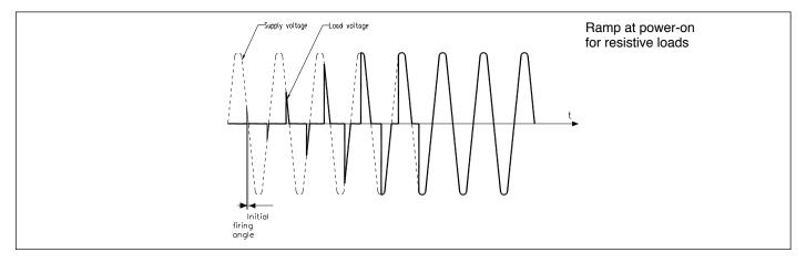
DT - Delay triggering" of first cycle (only for control modes ZC, BF mon-phase) Settable from 0° to 90°.
