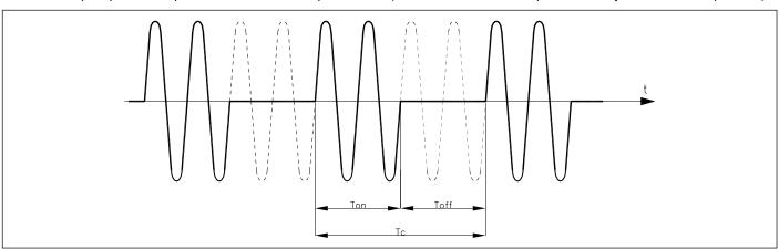
Example of operation in BF mode with power at 50%. A parameter defines the minimum number of conduction cycles settable (from 1 to 10). In the example, this parameter = 2.
