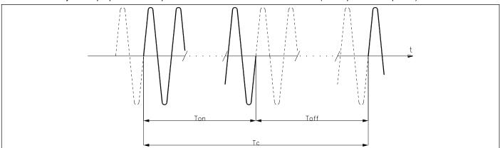
For example, if Tc = 10sec, if the power value is 20% there is conduction for 2 sec (100 conduction cycles @ 50Hz) and non conduction for 8 sec (400 non conduction cycles @ 50Hz).
