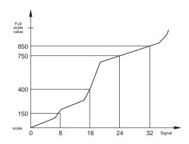
Positive polarization signals (eX. 0-50mV) St.0 is value displayed for minimum input (eX. 0mV); St.32 is value displayed for maximum input (es.50mV).
