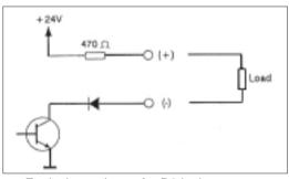
Equivalent scheme for D2 logic type output
