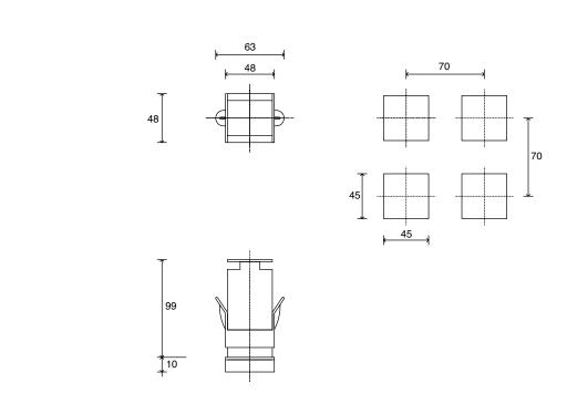
Dimensions: 48x48mm (1/16 DIN) depth 99mm
