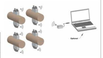
Very flexible system with 8 magnet sensors. Measures all tie bar diameters from 45.....>1000mm and even on flat surfaces, detects even cracks on tie bar, needs no steel bands or other mounting aids -> simple mounting with magnets in minutes.
